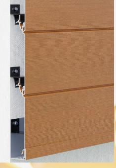
**STEP 4** Slide clips and screw into wall every 32 inches.
