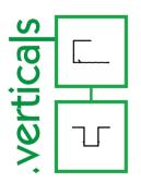
The LAP General J Trim: used for minor vertical delineation, doors and windows. Features the Easytrim ez.bump™, allowing horizontal fiber cement planks to nest inside the tab area creating an interior drainage channel.
