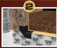
Remove release liner and apply the detail tape in each corner of the rough opening. Fold out over the BT25XL.
