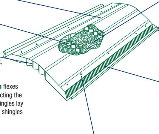
**Weather filter** provides advanced protection from rain, snow, dust and insect intrusion.
