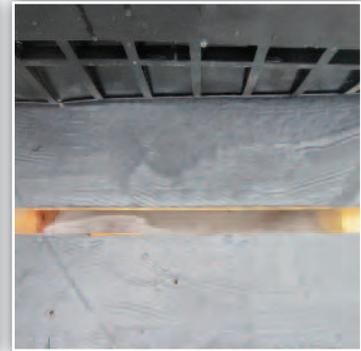
*During 30 days of freezing/thaw cycles, The Edge Vent was intentionally covered under an ice dam.*
