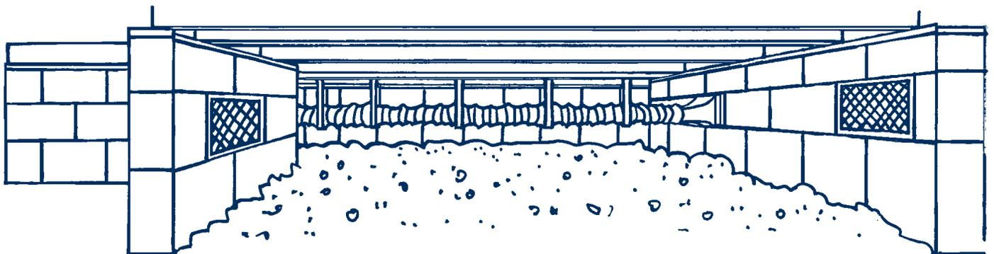
The powered duct system provides targeted ventilation to problem or hard-to-reach areas.
