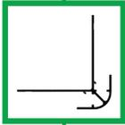
The **Rounded Outside Corner**: an alternate look to the square corner. Featuring the Easytrim **ez.bump™**, allowing the horizontal trim pieces to nest inside while keeping the panel flush to the tabs, creating an interior drainage channel.
