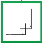
The **Inside Corner**: currently the only piece for trimming inside corners. Featuring the Easytrim **ez.bump™**, allowing the horizontal trim pieces to nest inside while keeping the panel flush to the tabs, creating an interior drainage plane.
