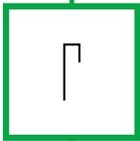
The **Soffit J**: used for finishing/capping the top of the system as required.
