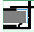
The **ez.bump™** allows the horizontal trim pieces to nest inside while keeping the panel flush to the tabs. This creates an interior drainage plane, flushing water away from the panels and wall.
