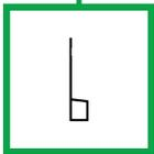
The **b Trim**: featuring the **ez.plane™**, using a 8 degree slope to drain water away from building. Used as an alternate to the Z Trim as the base horizontal trim where the underside is visible.
