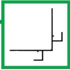
The **Square Outside Corner**: featuring the Easytrim **ez.bump™**, allowing the horizontal trim pieces to nest inside while keeping the panel flush to the tabs, creating an interior drainage plane.
