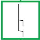
The **h Trim**: featuring the **ez.plane™**, using a 8 degree slope to drain water away from building. Used as the primary horizontal piece.
