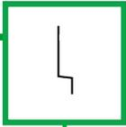
The **z Trim**: features the **ez.plane™**, using a 8 degree slope to drain water away from building. Used for the base horizontal trim, as well as above windows and doors.
