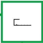
The **General J Trim**: used for minor vertical delineation, doors, and windows. Features the Easytrim **ez.bump™**, allowing the horizontal trim pieces to nest inside while keeping the panel flush to the tabs, creating an interior drainage plane.
