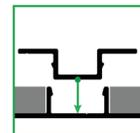
The **ez.lock™** system allows the primary verticals to be installed quickly and without fasteners. The top cap is tapped into place with a rubber mallet.
