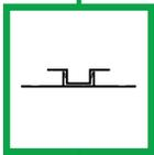
The **Panel to Panel Top Cap Vertical Top Cap / Back Plate Assembly**: Used as the primary vertical piece of the system. Features the Easytrim **ez.lock™** system, allowing the two pieces to snap together.
