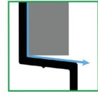
The **ez.plane™** feature creates a 8 degree sloped surface on the horizontal pieces that drains water away from the wall.
