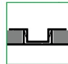
Once the top cap is fitted, the channel teeth will engage creating a secure lock.
