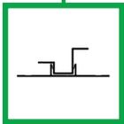
The **Panel to Plank Top Cap Vertical Top Cap / Back Plate Assembly**: Used as the vertical when transitioning from Easytrim Reveals System to lap siding. Features the Easytrim **ez.lock™** system, allowing the two pieces to snap together.
