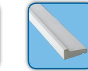
**Drip Cap**Used over a door or window to keep water from flowing under the cladding
